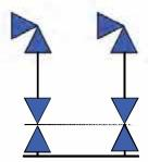
Interlocking block valve with two vessel penetrations
