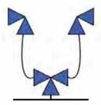
Three way block valve with pipe elbows
