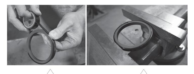
Figure 21 Model 361 Piston Ring Vise Break Method (Step 1)
