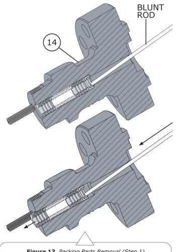
Figure 13 Packing Parts Removal (Step 1)
