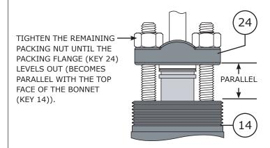
Figure 27 Double PTFE V-Ring Packing Tightening Diagram
