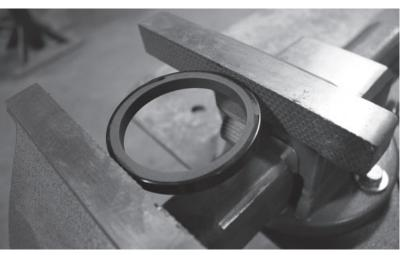
Figure 20 Piston Ring Assembly for Model 391 Valves (Step 1)
