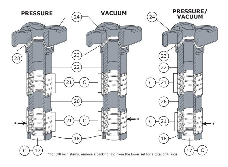
Figure 28 390 Series Control Valve PTFE Packing Diagrams
