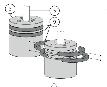
Figure 11 Model 391 Piston Ring Removal
