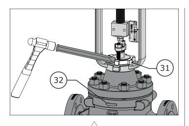
Figure 4 Yoke Nut being loosened with a Chisel
