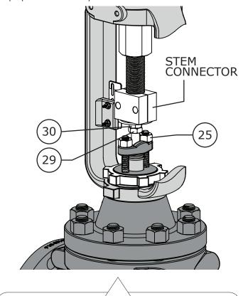
Figure 5 Packing Nut and Stem Connector Detail
