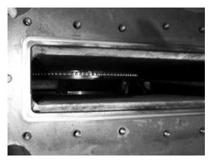
**6.1.11** Clean and inspect the seat pockets in the valve body. A cleaning tool can be made from a piece of rod or barstock. File a tapered edge on one end of the rod. Bend the tapered end to 90° and use it to clean the seat pockets of sludge or debris.
