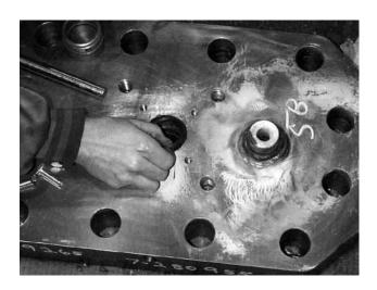
**5.3.15** Remove the T-bar from the new stem.
