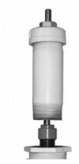
**5.3.6** Remove bonnet nuts. Studs may also be removed, if desired, to allow more work clearance.
