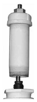
**5.6.6** Remove bonnet nuts. Studs may also be removed if desired to allow additional work clearance.
