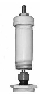
**5.1.6** Remove bonnet nuts. Studs may also be removed if desired to allow more work clearance.
