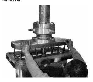
**5.8.7** Using proper equipment and lifting procedures, lift the entire top works assembly, bonnet, cupola, and gate high enough to clear the T-bar slot in the gate. Insert customer supplied drift pins in the holes provided in the bottom of the gate T-bar slot.
