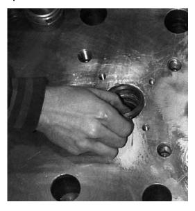
**5.6.18** Clean, inspect, and install the bolted stem packing retainer. The upper adapter ring of the stem packing should seat in the counterbore located in the bottom of the bolted stem packing retainer. Fasten to the bonnet using capscrews. DO NOT tighten capscrews at this time.
